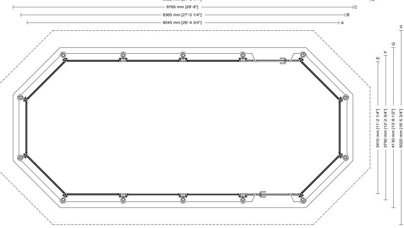
B Column axis C Foundation base D Roofing E Internal windowsill F Column axis G Foundation base H Roofing
