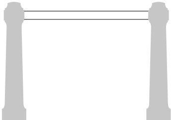
Tube 9522.842 Accessory for railings per linear meter • Painted hot dip galvanized steel • Ø 42mm x 3mm of thickness
