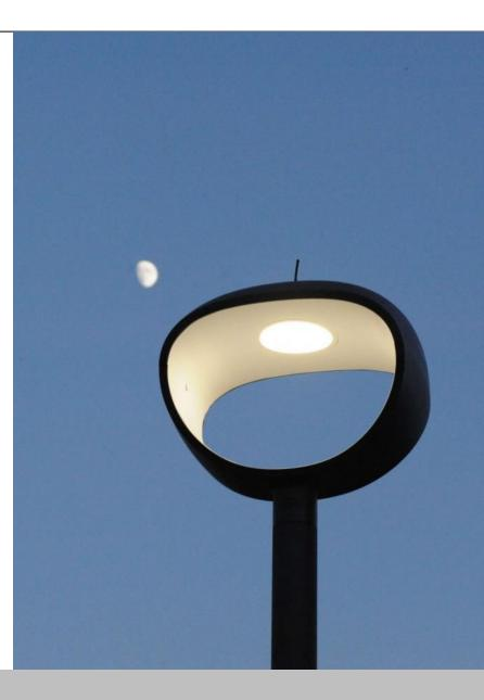
Hydra is equipped with blue LEDs and a glass treated with remote phosphor: when the blue light passes through the glass it assumes a warm white tone
