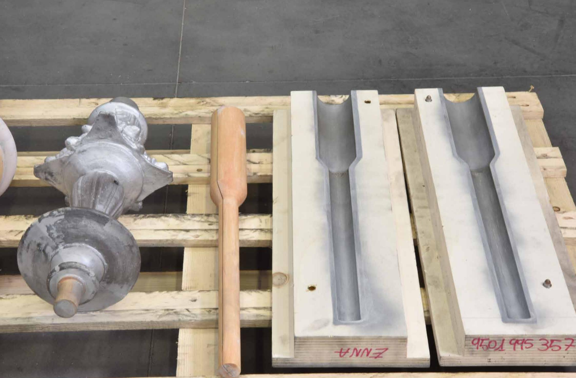
The patterns and the corresponding cores made new castings possible in the foundry. A manual job calling for great care and precision.
