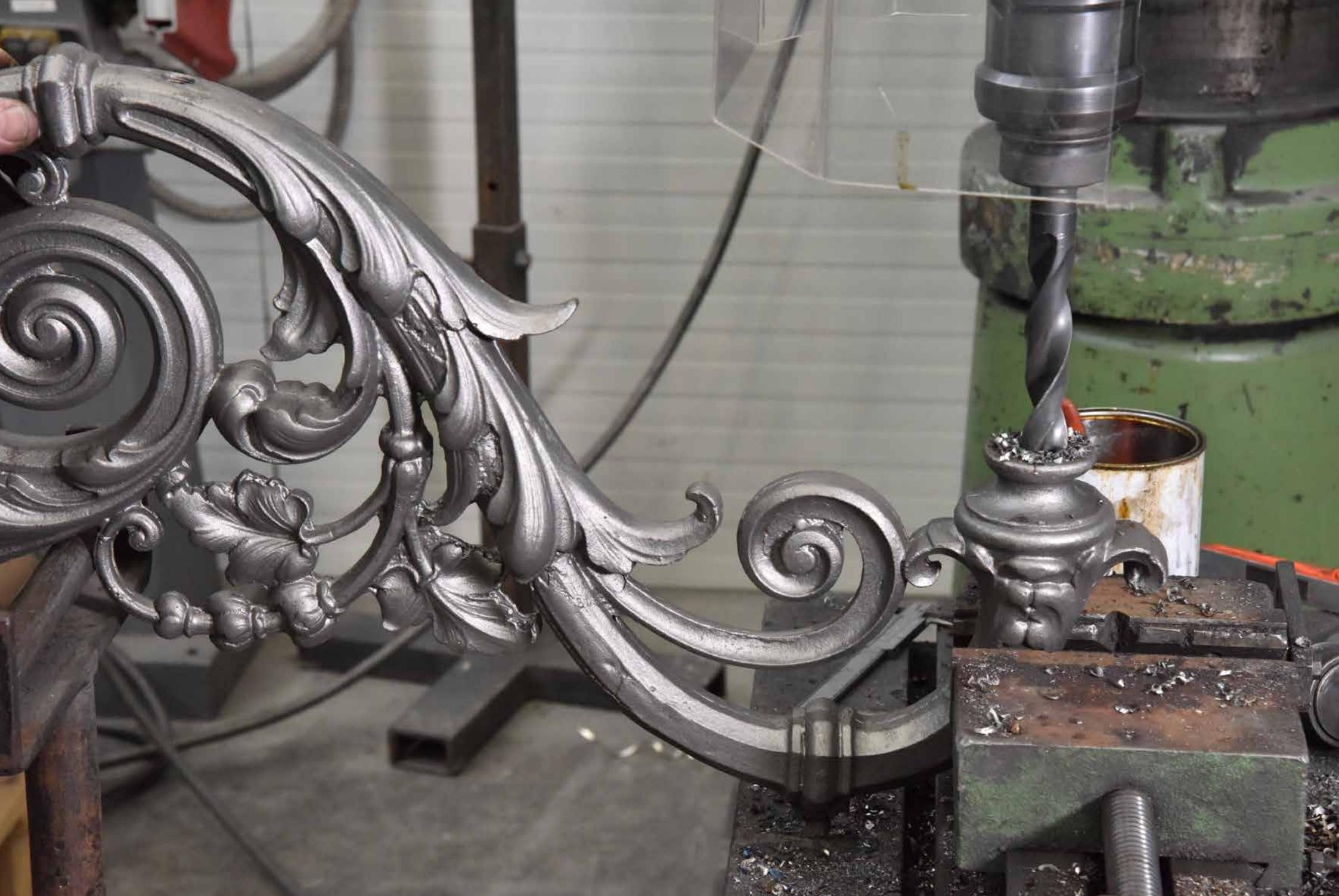
After the mechanical reconstruction operations, all the individual cast iron components were once again sandblasted and puttied in preparation for the painting.
