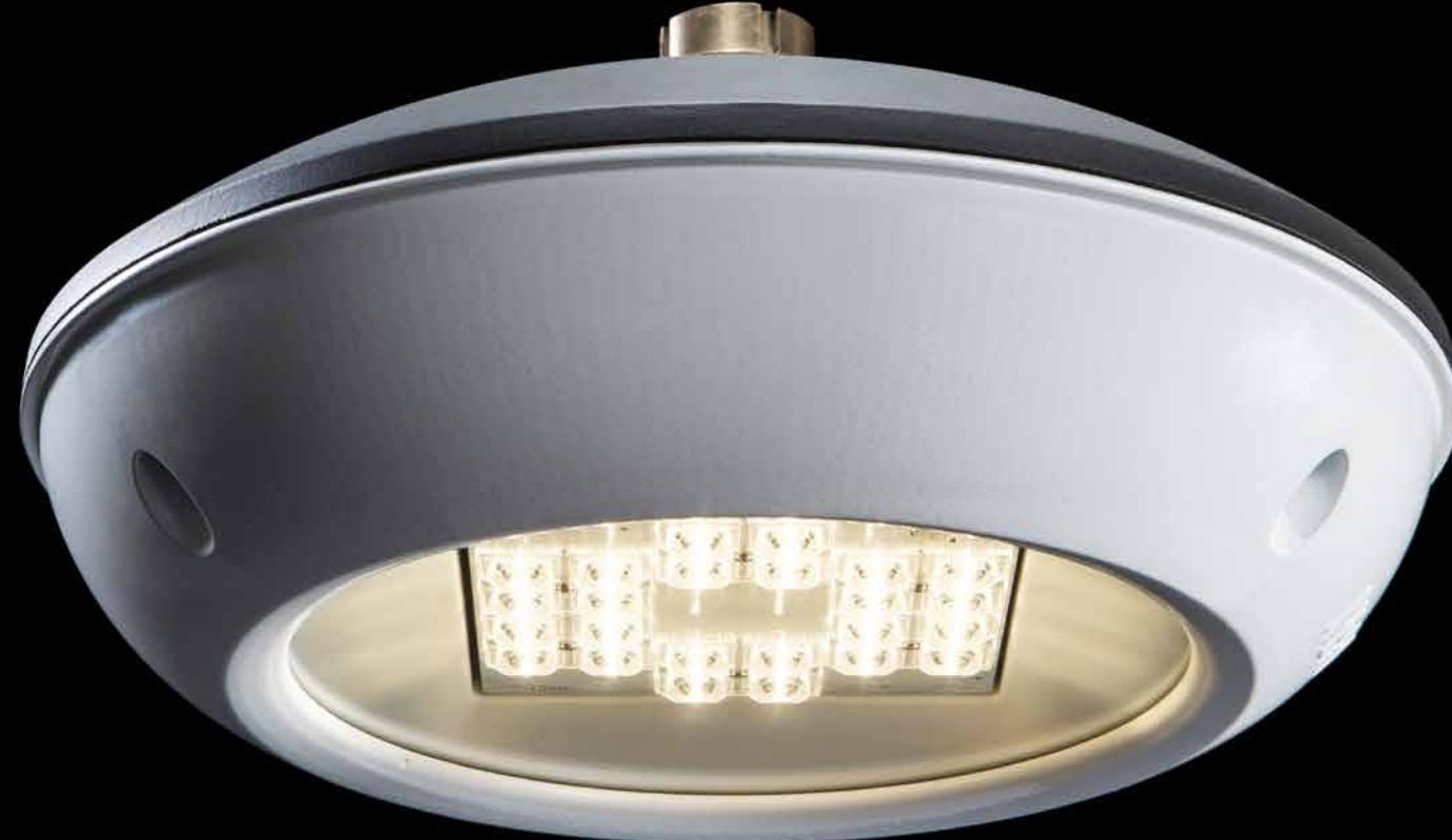
The body entirely made in cast aluminium and extra-clear transparent glass is equipped with an upper frame in Neri Grey, whereas the lower frame is white in colour. The large internal dimensions allow for optimal irradiation dissipation thanks to the new anodised dissipater. The LED module can be removed easily as it uses the new fast demounting system which does not require the use of tools, unless when disconnecting the isolator switch cables.
