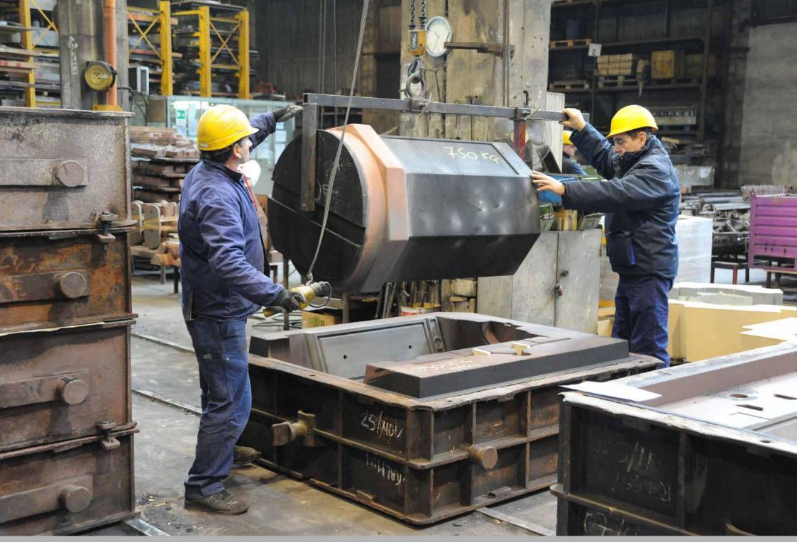
It is a very delicate passage. The precision with which the core is positioned directly determines the quality of the casting.
