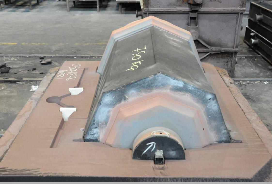
The two earthen moulds are then combined by superimposing the empty one to that containing the 'core'.
