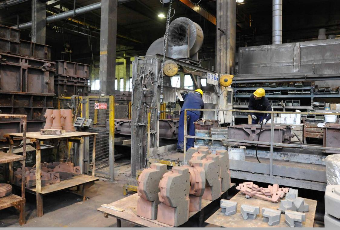
Now the two shapes aligned on the ground are prepared for the positioning of the 'inner core'.
