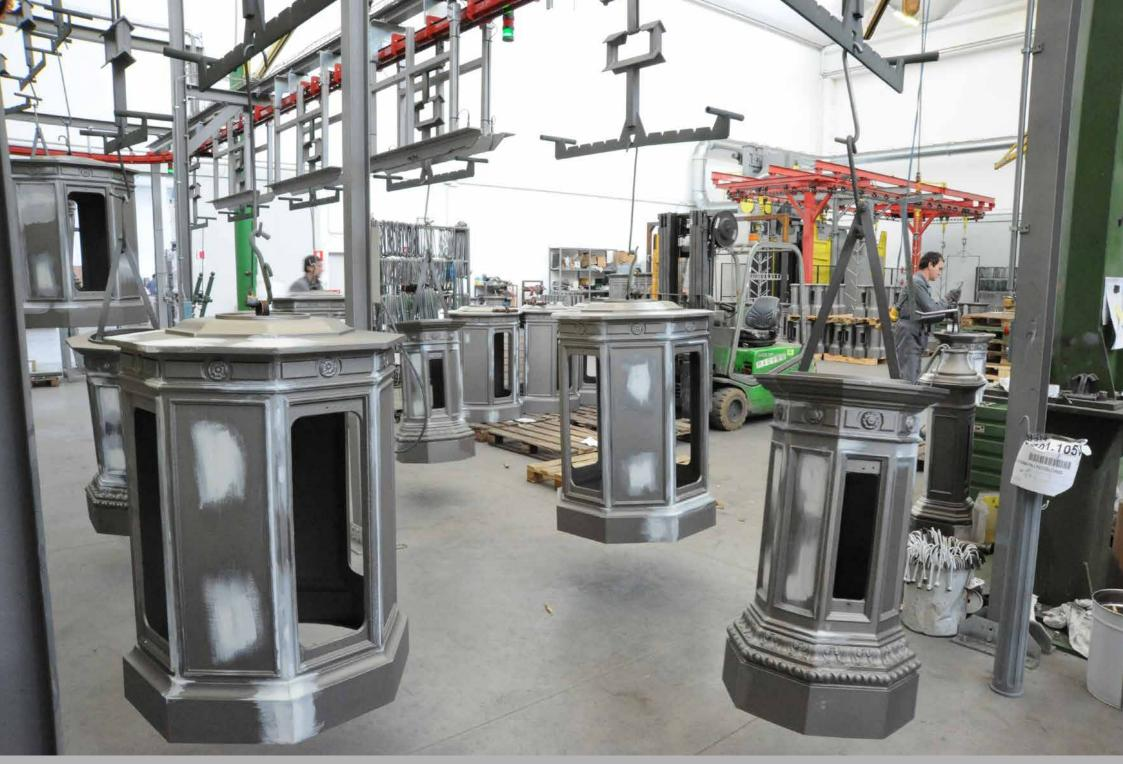
All bases are dipped in a large tank containing liquid galvanising zinc, capable of protecting the cast iron from rusting both inside and outside.
