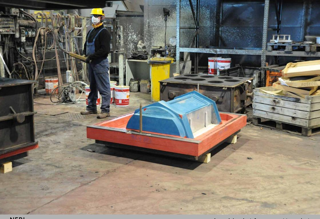
... and is treated with special coatings that will improve the detachment of cast iron from the sand.
