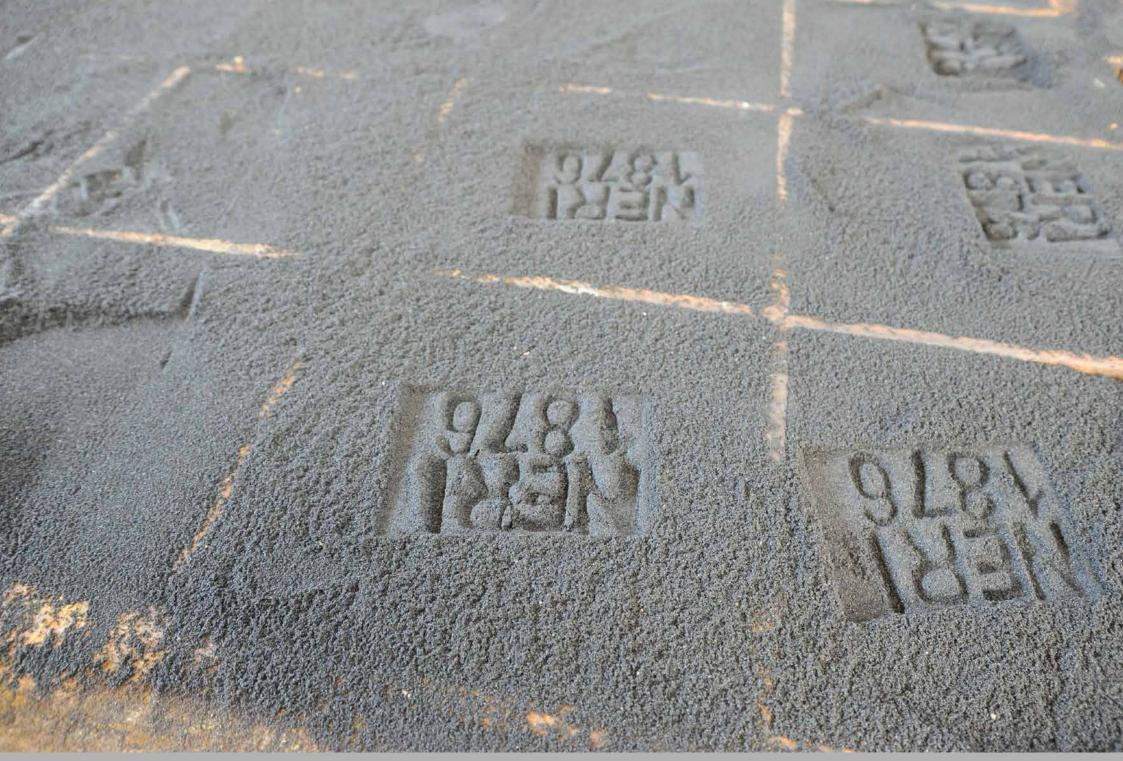
The shape impressed in the resin-sand (mould) is then separated from the model...
