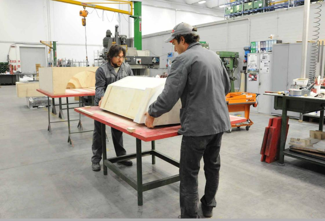
A similar model is made to produce the 'core', a necessary element to create the inner cavity.
