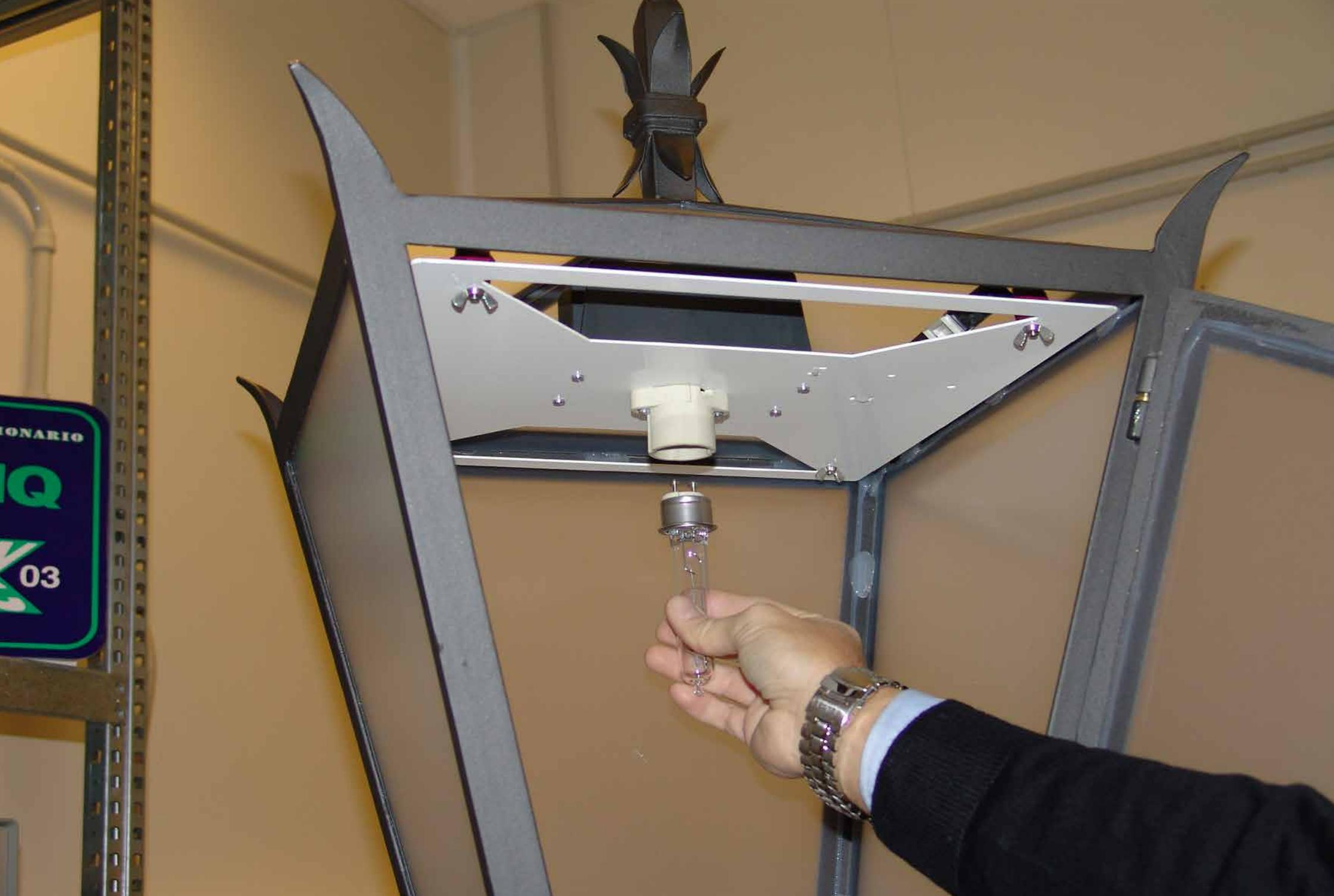
The passage from 125 W mercury lamps to latest generation Philips CPO-TW 60W (2800K) light sources has produced a 65% reduction of electrical power consumption with a simultaneous increase in light on the ground. The photometric results obtained in the laboratory have been certified with the IMQ Performance mark. Light pollution (upward emissions) was reduced to 25.70% ULOR
