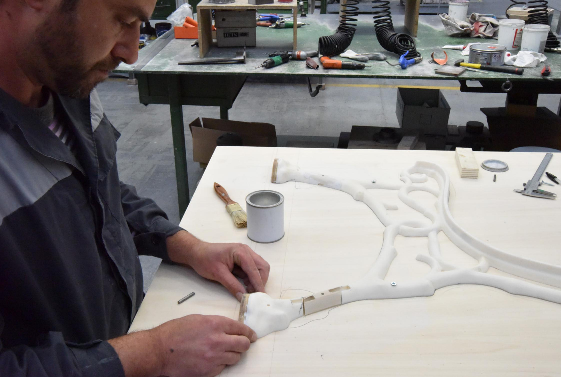
With the new longer mould, we replicated all of the operations described above, to create two models for casting the bench in its new longer version.
