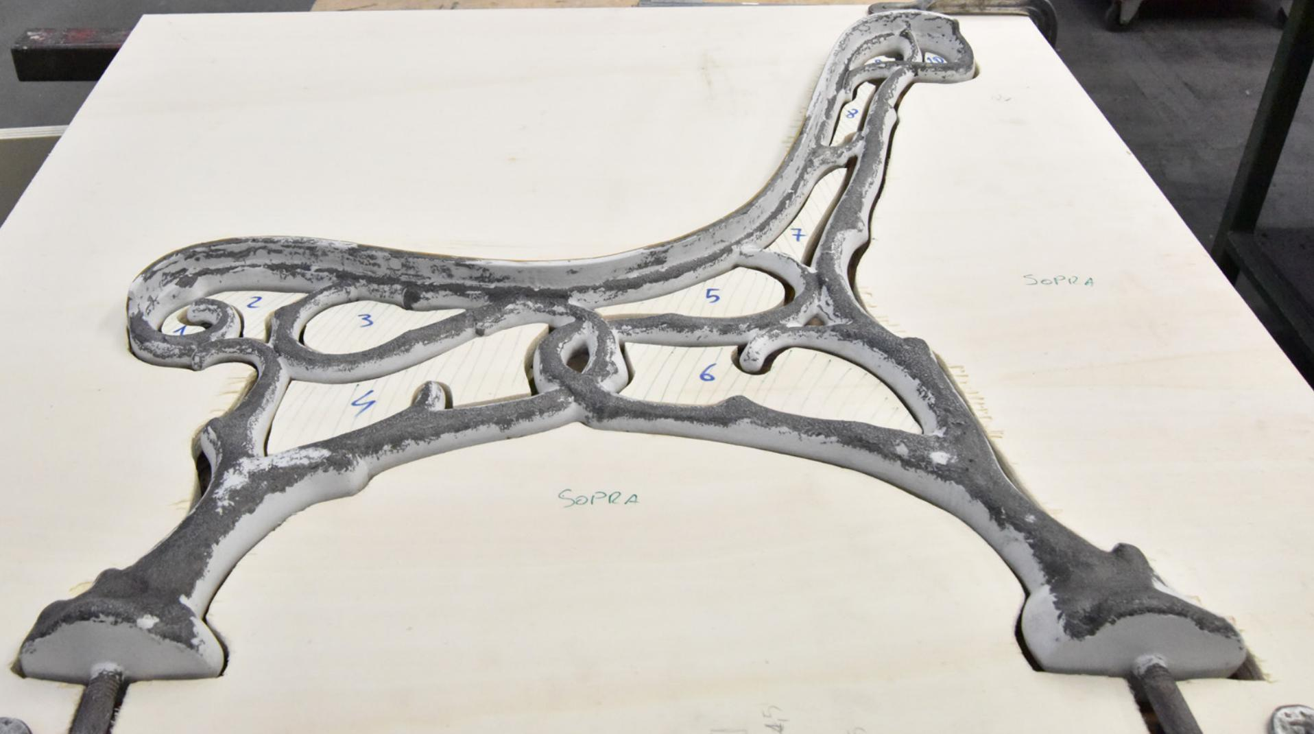
All of the spaces between the wood and the original cast iron model were then sealed with putty. The part in cast iron that was outside the wood corresponds to the exact half of the bench.
