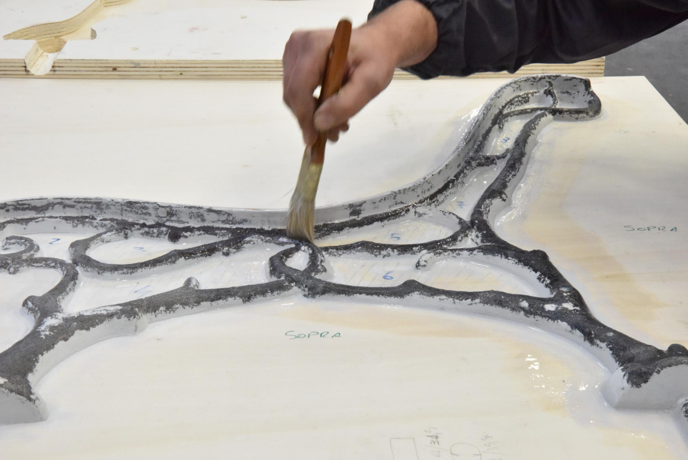
Then, we used hand tools to make a wooden model that is perfectly specular to the type of bench that we were working with.
