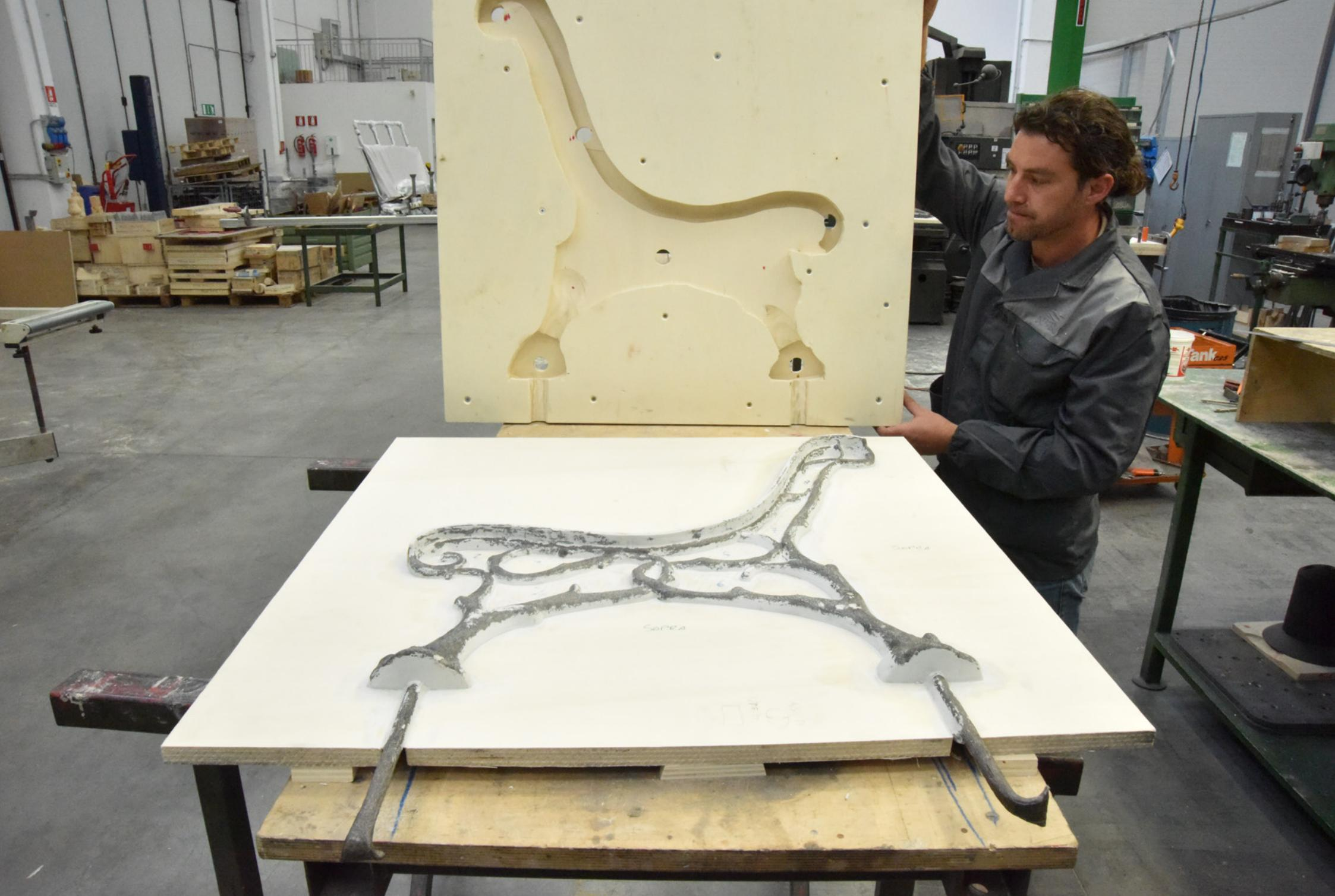
This model was then placed over the prepared bench and we poured resin into it to reproduce the original form and create the desired mould.
