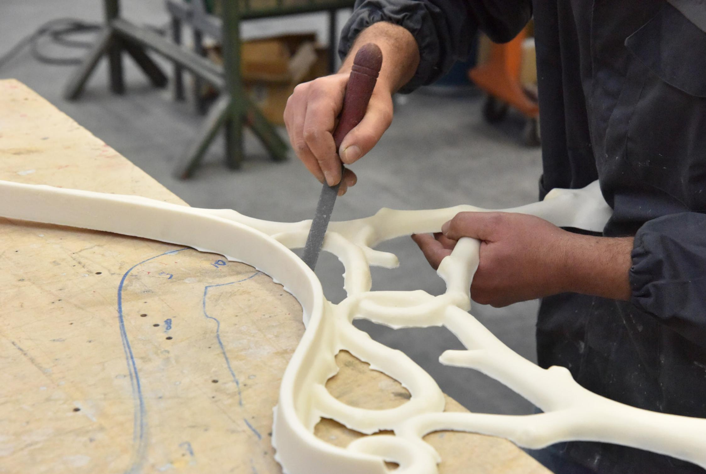
The height of the original bench, declared insufficient by designers, was modified to improve ergonomics. Here at the Neri factory, we adapted the resin model to lengthen the base.
