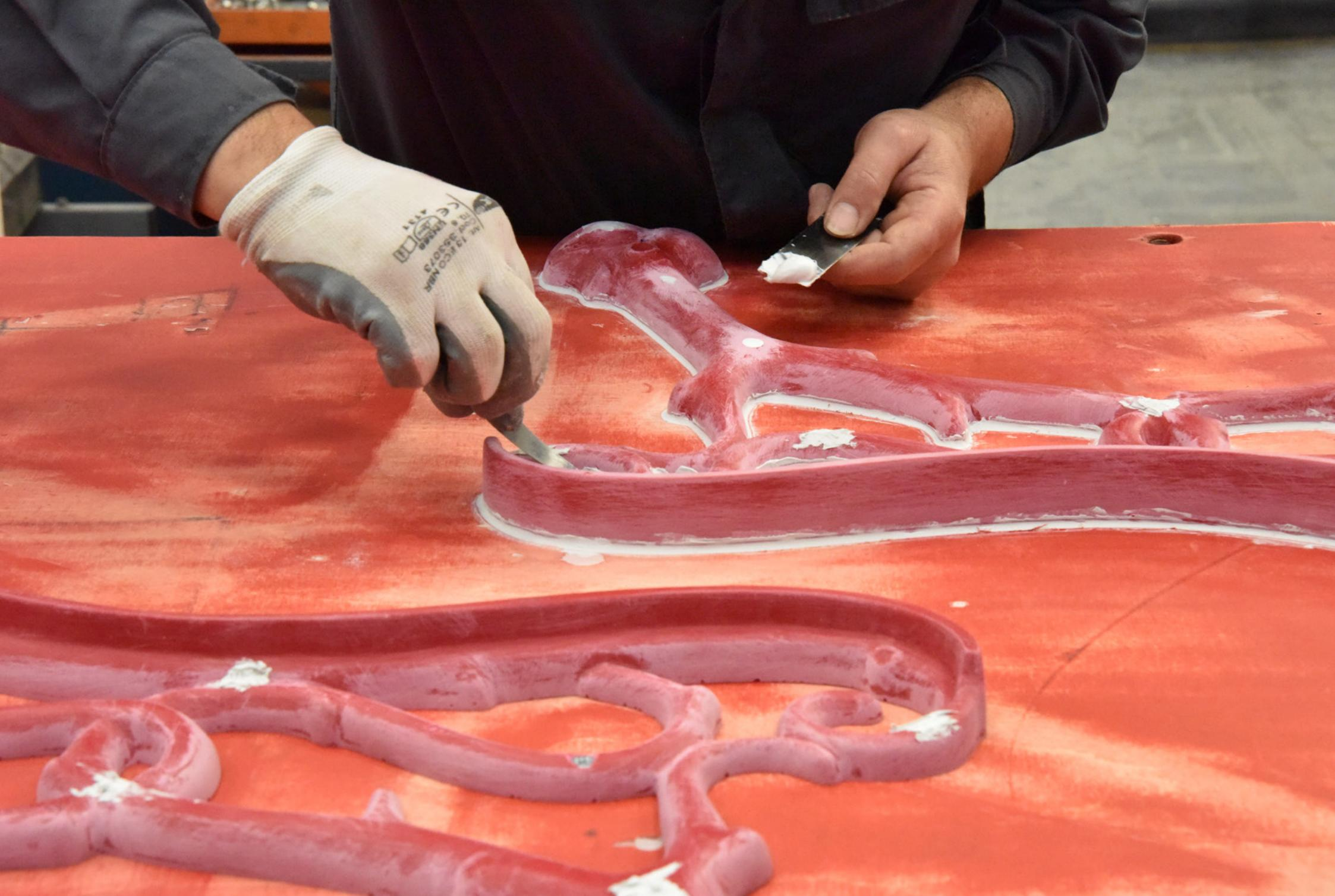
On the plate, various wood plugs were also fitted to correspond to the pours where the cast iron flows to reach all of the surfaces.
