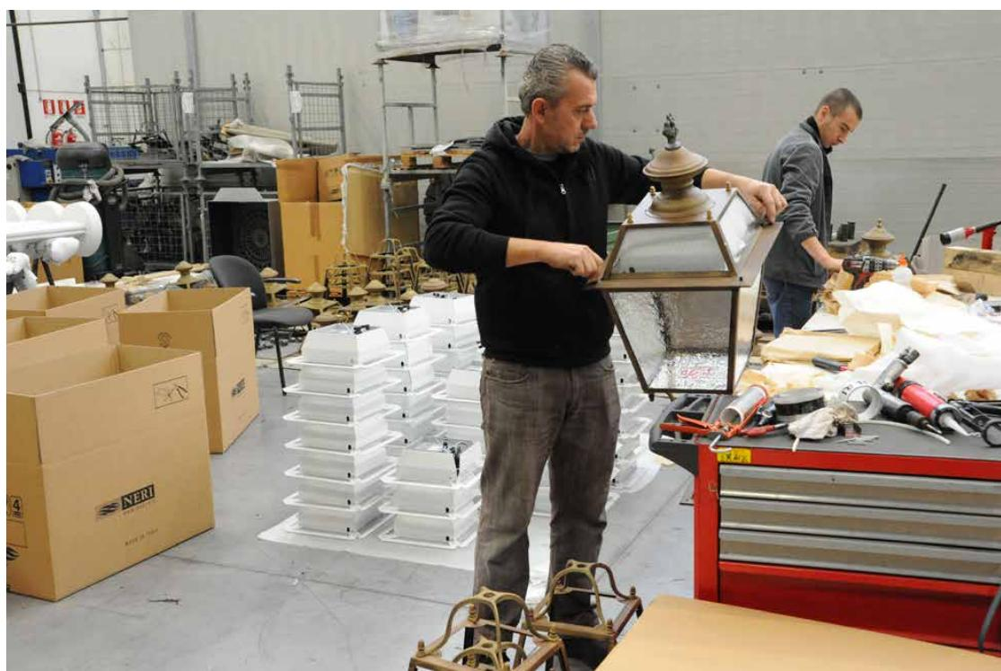
In the original lantern, before the intervention, light reflected on the walls and above the lantern. Even though the intention was to reduce this effect and the resulting skyward light dispersion, it has been agreed to keep a partial orientation towards the upper part of the lantern to preserve Florence's characteristic nocturnal atmosphere and to fully appreciate the shape of the lamp.
