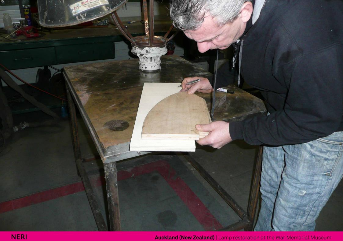
With the wooden mould, it was possible to bring the various frames back to their original shape.
